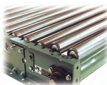
POP-OUT ROLLERS (some rollers raised for clarity)
